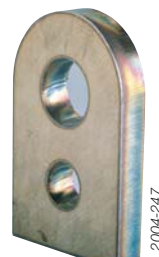
HP cut - 15mm stainless steel ArH 2 /N 2
