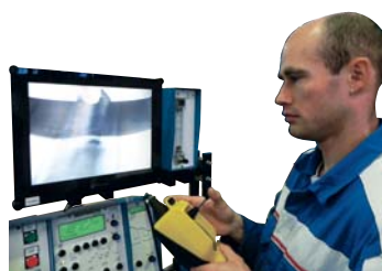
System with large color screen 15", miniaturised camera and additional lighting
